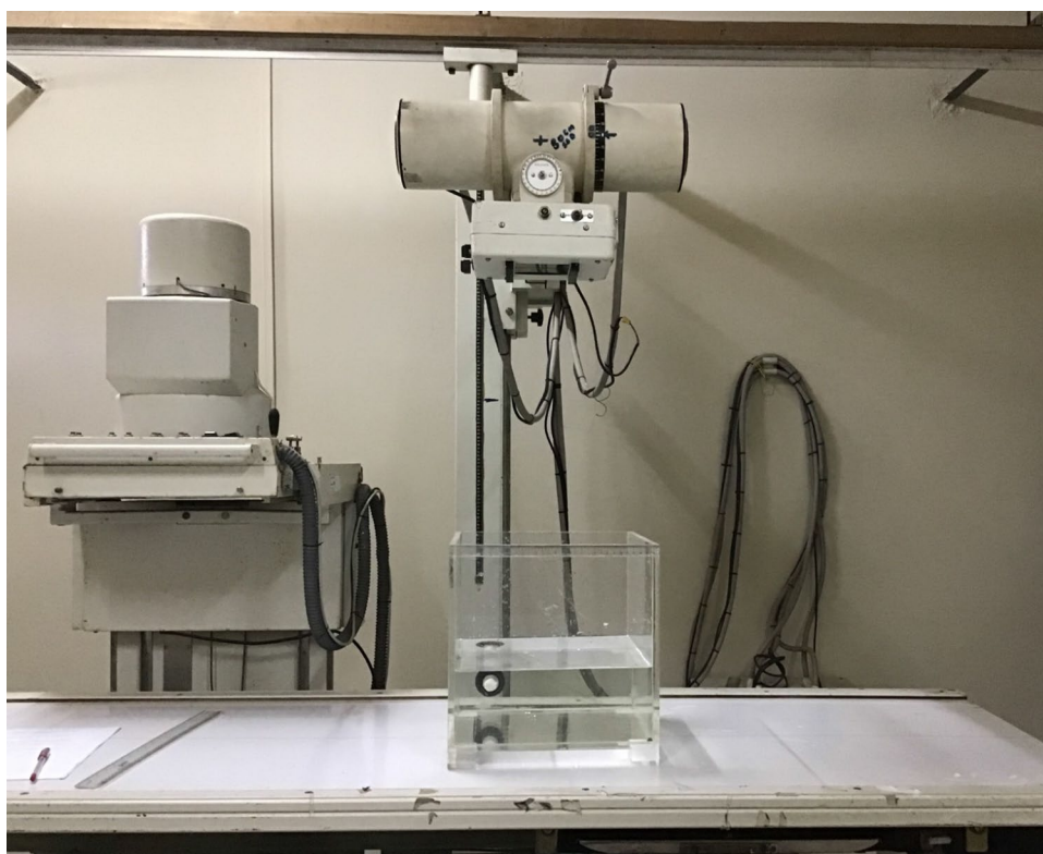
Fig. 3 A water phantom setting to measure stray radiation for vertical exposure (couch mission)
