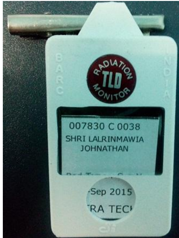
Fig. 3.2.5: Thermo-luminescent dosimeter used to measure radiation dose of the investigator
