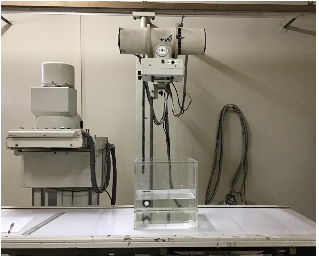
Fig. 3.5 (b): A water-phantom setting to measure stray radiation for vertical exposure (couch mission)
