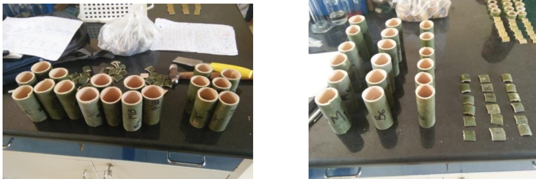
Figure 3.3 Samples for shrinkage and swelling test
