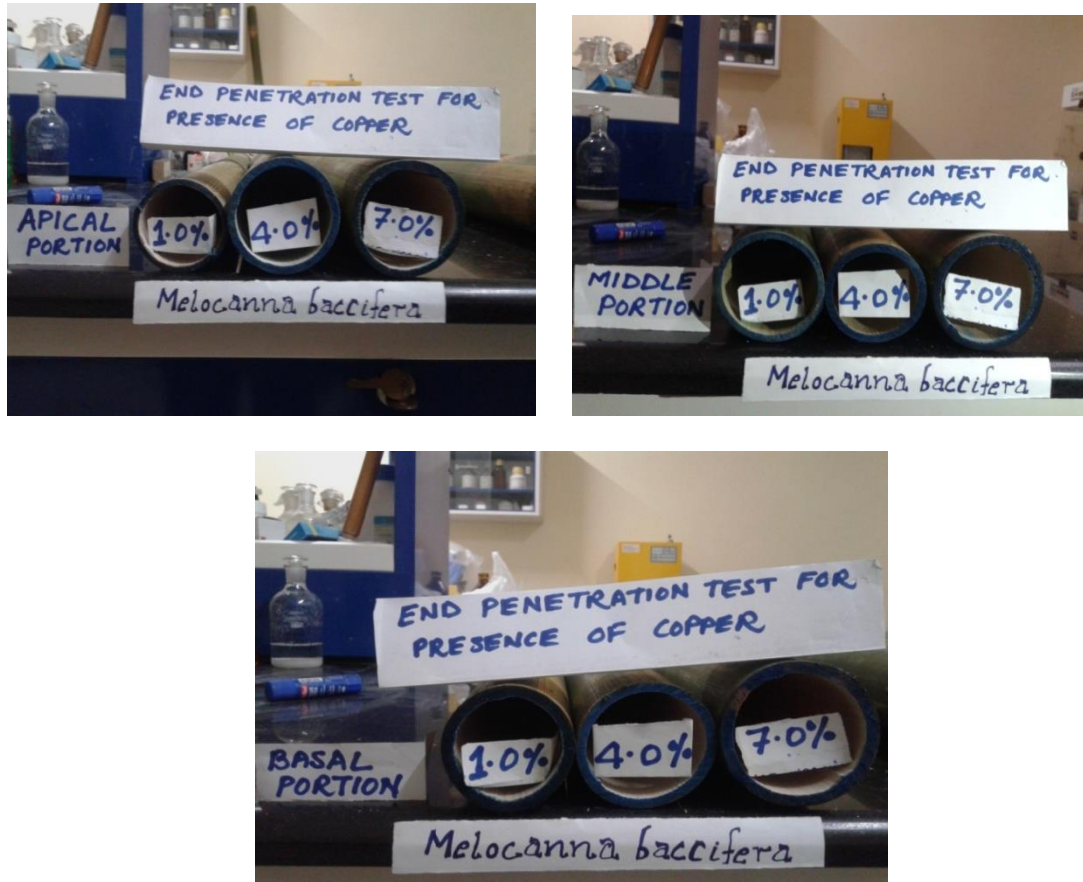
Figure 4.3 End penetration test for copper in three portions of bamboo
