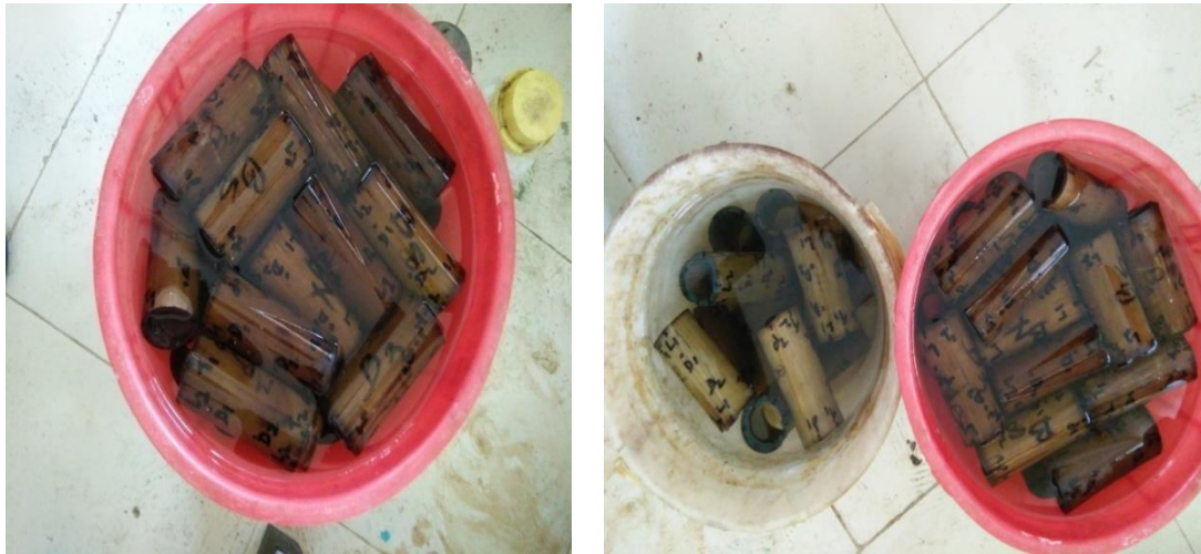
Figure 3.4 Immersion of samples in water for volumetric swelling
