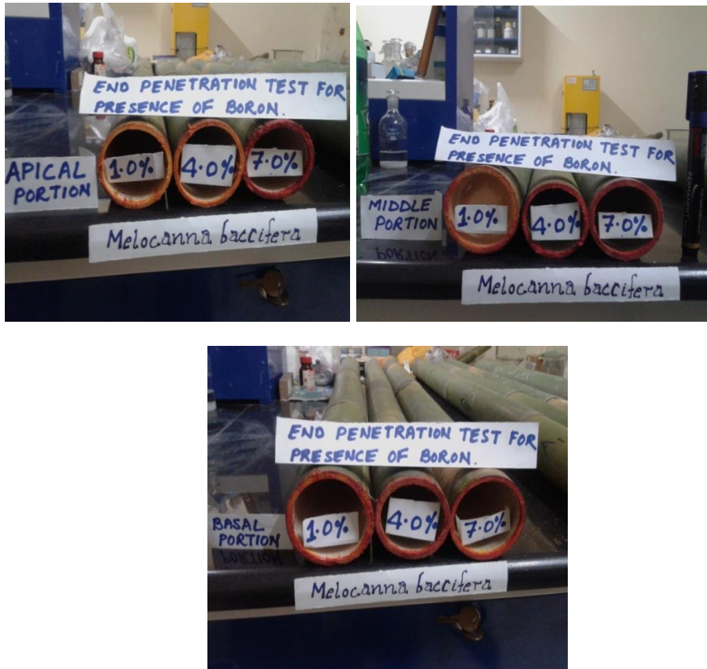
Figure 4.4 End penetration test for boron in three portions of bamboo
